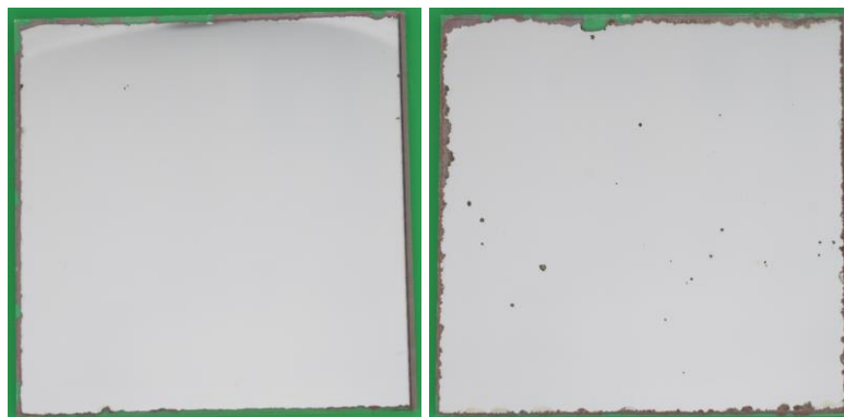
Figure 23. Photograph of leaded-containing sample (left) and lead-free sample (middle) after 36 months of exposure in Almería.
