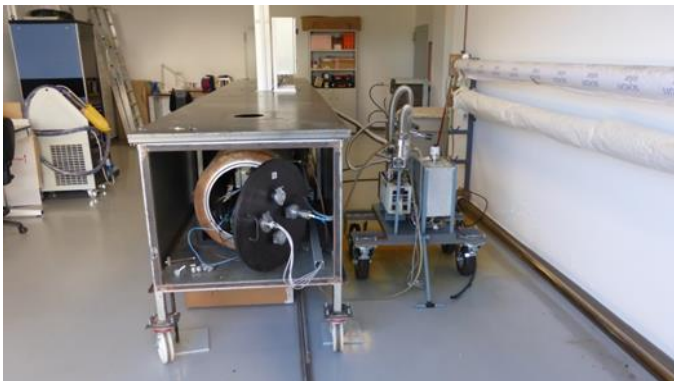
Figure 108. View of the HEATREC test chamber to measure heat losses in solar receiver tubes (left) and RESOL test bench to measure the receiver's optical efficiency (right).
