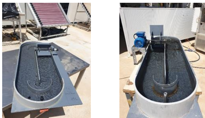
Figure 89. Raceway Pond Reactor with capacities of: a) 15 L and 5 cm of liquid depth and b) 90 L and 15 cm of liquid depth.
