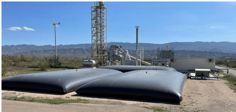
Figure 84. Containers filled with real seawater for desalination tests in closed loop.
