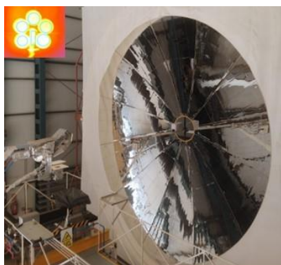
Figure 25. Test bench for silicon carbide (SiC) accelerated ageing at CIEMAT-PSA's SF40 Solar Furnace, with improved reflective surfaces. (Left corner) Infrared image of SiC samples at 1,200 °C
