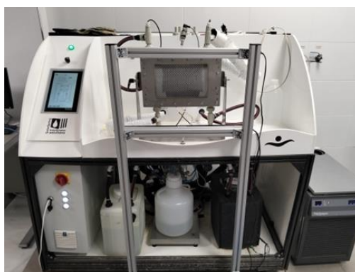
Figure 120. Bench-scale unit for testing MD with flat-sheet membranes (left), and UV-A arrangement for wetting characterization (right).
