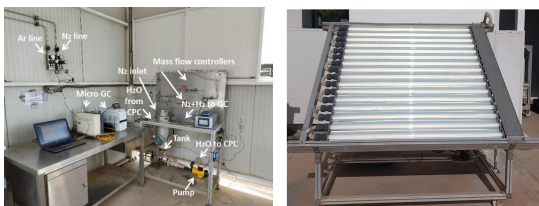
Figure 97. Photoreactor installed at PSA-CIEMAT facility composed by: (left) Stainless steel tank, mass flow controller and gas cromatograph and (right) Compound parabolic collector (CPC).
