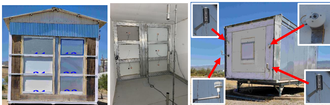
Figure 42. Tested panels installed in the CESPA III and PASLINK Test Cells where they were tested. (left) Identification of the panels tested at CESPA III Test Cell, (centre) sensors installed in the indoor surface of the panels and Test Cell, (right) panel installed in PASLINK Test Cell and sensors measuring climate variables.
