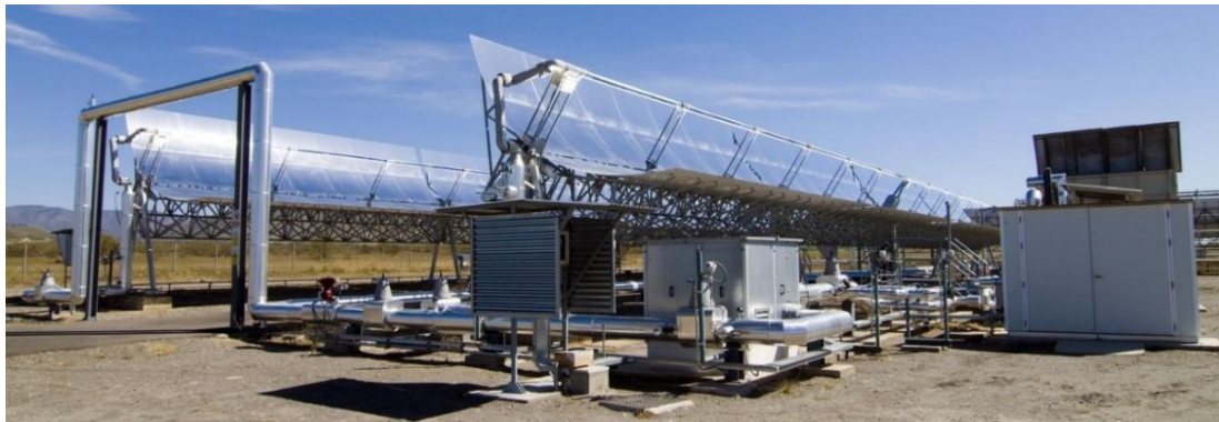
Figure 53. View of the IFL experimental facility (with parabolic troughs) using compressed gas as heat transfer fluid.
