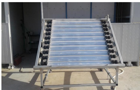
Figure 87. View of 2 m 2 -CPC coupled to Electro-Fenton pilot plant (ELECTROX).
