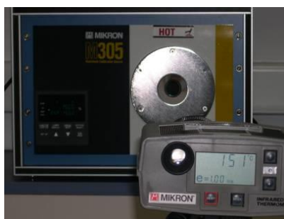
Figure 111. IR sensor calibration using a black body.
