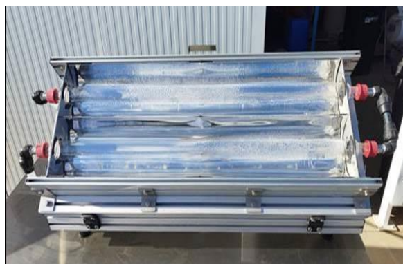
Figure 34. Final prototype CPC photoreactor constructed in SolarChem 5.0 project.
