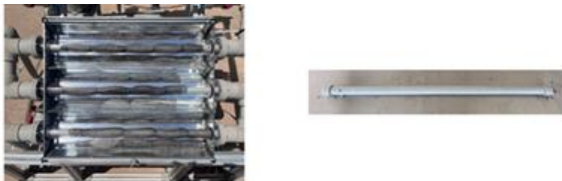
Figure 37. New solar photoreactor for testing supported photocatalysts to test both oxidation and reduction capacities. Left: CPC photoreactor with the supported zero valent iron in a mesh inserted in the tube thanks to the polypropylene support used. Right: one tube.
