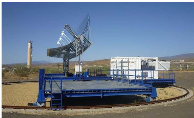
Figure 56. Side view of KONTAS test bench and the heating/cooling unit (right side).
