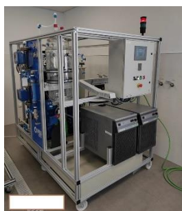
Figure 102. MD + crystallizer pilot plant developed by Apria Systems S.L.
