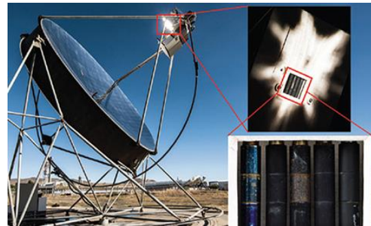
Figure 70. Accelerated aging tests of steel samples at a parabolic-dish DISTAL- II
