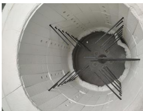
Figure 67. Picture taken from the top of the tank, showing its internal room and thermocouples at different lengths and radial positions.
