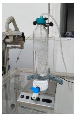
Figure 104. UV-transparent laboratory tubular reactor available at PSA facilities.
