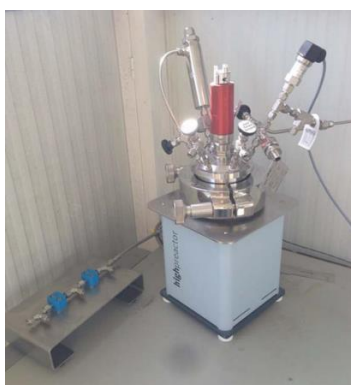
Figure 98. Wet Air Oxidation Pilot plant.
