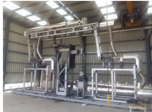
Figure 57. Schematic diagram of the REPA test loop at PSA (left) and north view of the test facility with two flex-hoses mounted for testing (right).
