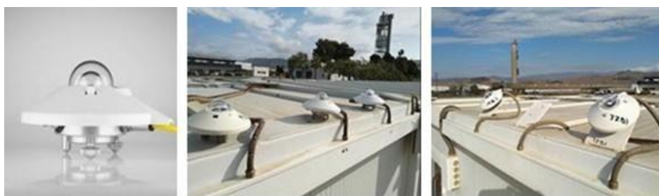
Figure 100. CUV-5 radiometer (left). View of all solar UV radiometers, horizontal (centre) and inclined (right) setup used in the Solar Treatment of Water Unit.
